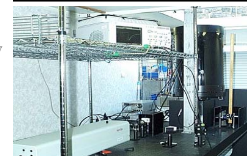
The Mobile laboratory houses the Lidar system.
